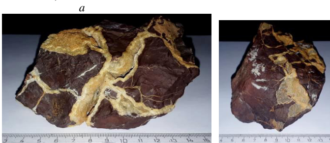
Fig. 1. Bauxite fragment (with calcite depositions) collected from Lonea I waste dump: a – front view; b – side view)
