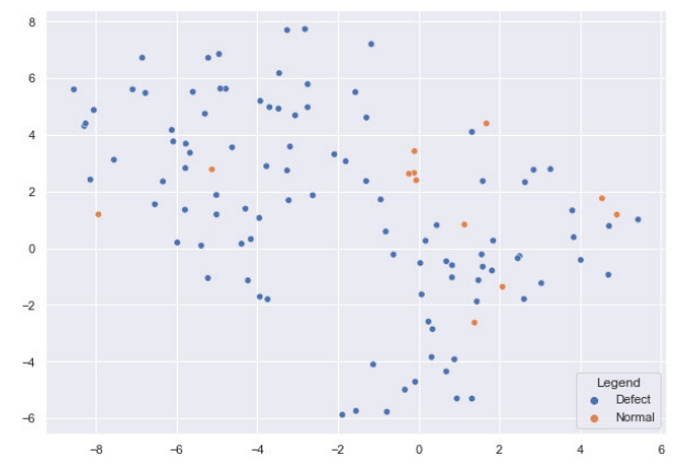
Figure 11. Visualization of derived bearing signal spectrum statistics
