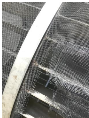
Fig. 1. The rupture site of the titanium mesh
