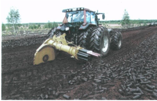
Fig. 3. Extraction of lump peat by the milling method
