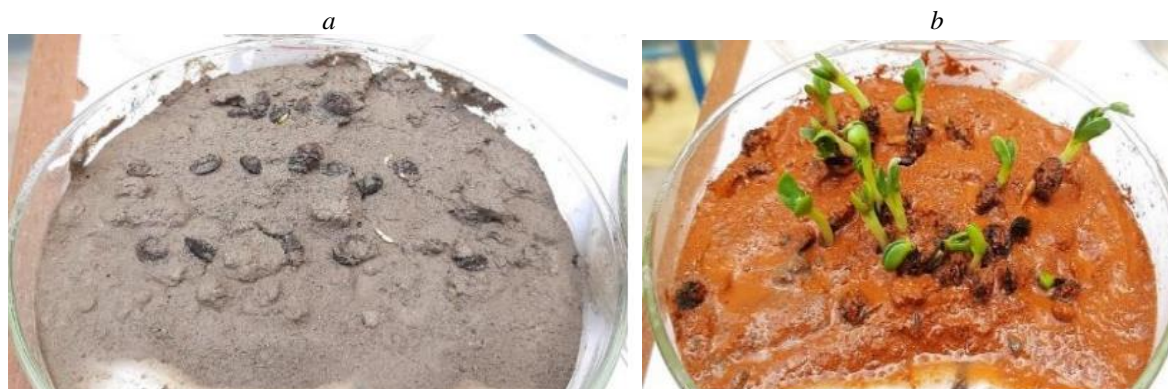
Fig. 3. Germination of alfalfa on oil-contaminated soil before (a) and after treatment with 0.1 wt.% Rau-85 + 0.5 wt.% solution of organomineral biofertilizer (b)
