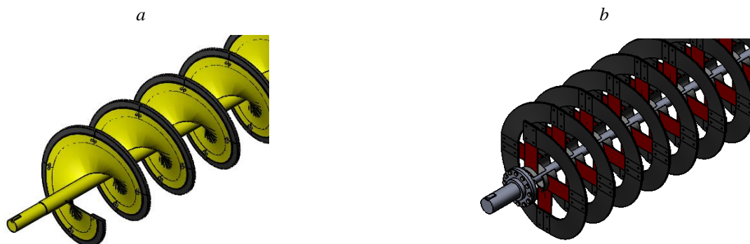
Fig. 3. Screw classifiers screw: a - basic; b - modernized
