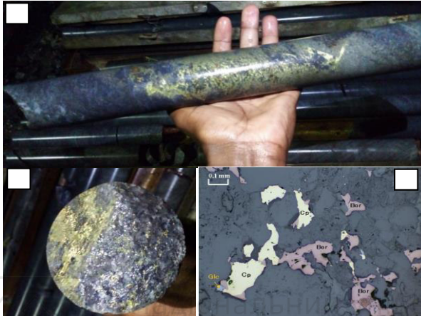
Fig. 3. Showing Bornite(dark blue) & Chalcopyrite(yellow) mineralised C - Quartzite(C-Orebody) from 61P5 1523 mL; (A) Longitudinal 49 mm diameter core sample, ( B) Cross-sectional view of the 49 mm core sample, (C) Thin section of the C-Orebody sample
