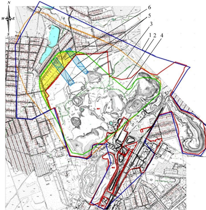
Fig. 3. Formation of the shear zone and the new land use within its boundaries for subsoil use needs at the Ternivska mine, the JSC Kryvbaszalizrudkom : 1 – boundaries of the mining allotment of the Ternivska mine; 2 – boundaries of the land allotment of the Ternivska mine; 3 – design boundaries of the earth surface displacement zone when mining naturally rich iron ores without leaving pillars, level 1350-1500 m, the Ternivska mine (option I of the feasibility study); 4 – design boundaries of the earth formation according to option II of the feasibility study accepted for further deposit mining, the Ternivska mine
