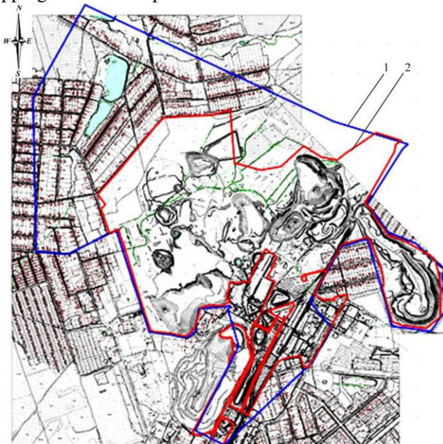
Fig. 1. Surface plan of the Ternivska mine of the JSC Kryvbaszalizrudkom: 1 – mining allotment; 2 - land allotment
