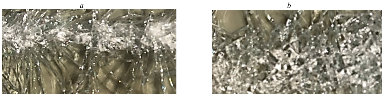
Fig. 2. Fragments of destruction of the glass component of the triplex upon contact with the impactor: a - shock loads on the material; b - shock and shear loads on the material
