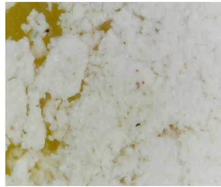
Fig. 2. Non-magnetic product x200 Results of X-ray phase analysis of enriched kaolin samples. XRF analysis was performed on a DRON-2 X-ray diffractometer in monochromatized Co-K \alpha radiation ( \lambda=1,7902\text{\AA} )
