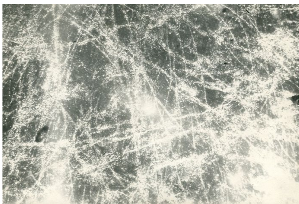
Fig. 1. Four systems of microdeformations in quartz grain of carboniferous sandstone of the Donetsk-Makeevsky region of the Donetsk basin
