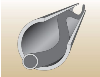
Figure. 1 Contact of the bent part of the drillstring with the cylindrical wall of the well
