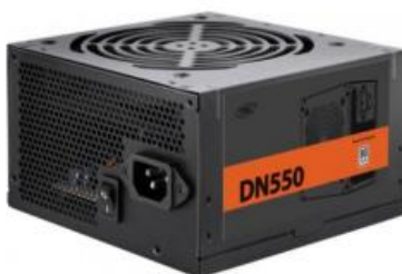
Figure 4.3 – External appearance of the computer power supply unit.
