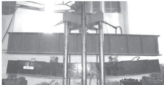
Fig. 2. The typical deflection and cracking pattern of composite steel beam strengthened with steel plate
