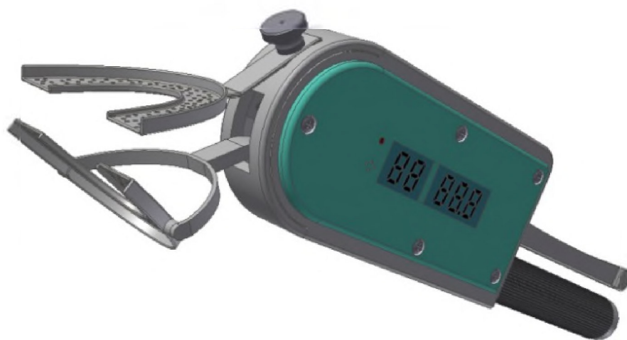
Fig. 1. Appearance of the device of own design for dosed active-passive mechanic therapy of mandibl
