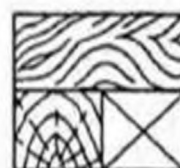
WOOD WITH GRAIN CROSS GRAIN; BLOCKING
